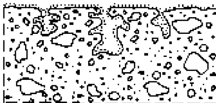
Figure 1 — Schematic drawing of a typical hydrophobic impregnation
