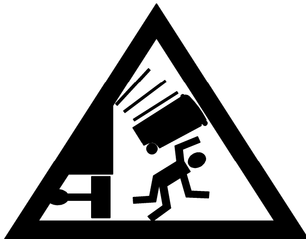
Figure B.6 — Warning sign: Falling container or object
