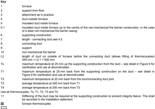
Figure 6 — Non-mechanical fire barrier mounted remote from the standard supporting construction and inside the furnace
