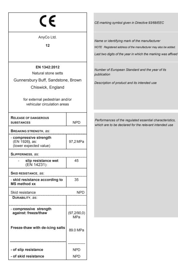
Figure ZA.1 — Example of CE marking on a packaging of setts of natural stone
