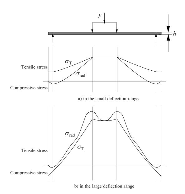
Figure 1: Schematic dependence of radial and tangential stresses upon the radius of the specimen, when loaded by a double ring device
