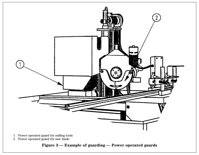
The interlocking devices with and without guard locking shall comply with the requirements of EN 1088:1995. In particular for machines where the maximum run-down time is 10 s or less, guard locking shall be achieved by at least an interlocking device with manually operated delay device as shown in, EN 1088:1995, Table 1.
