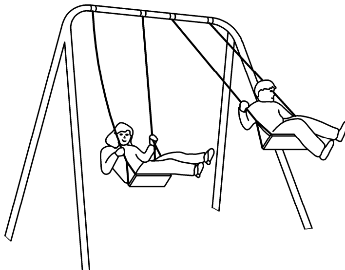
Figure 1 — Example of a swing with one rotational axis (Type 1)
