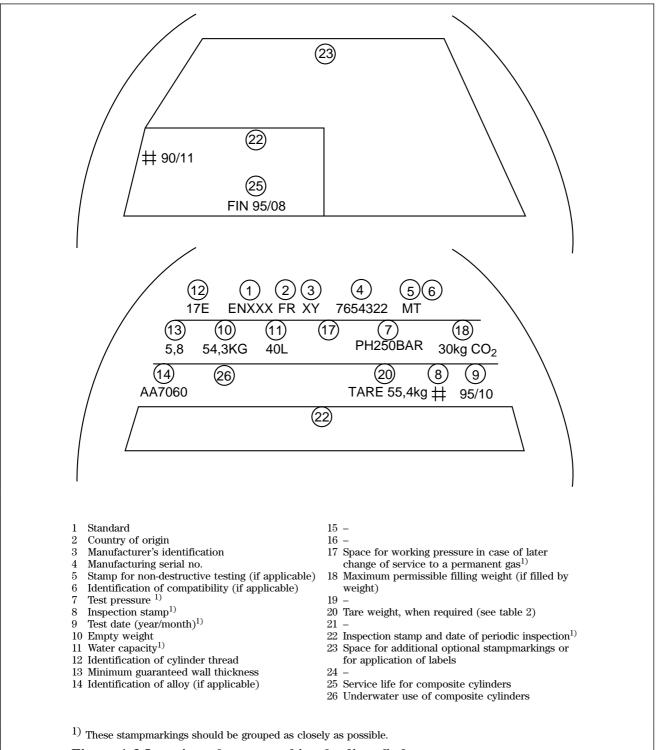
Figure A.2 Location of stampmarking for liquefied gases
