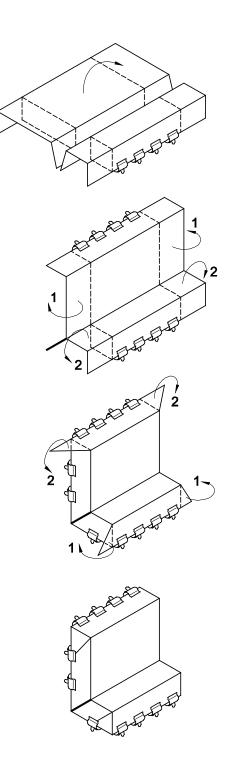
**Stage 1**: With test rig opened out flat and fillings in position, thread cover behind hinge pin and clip to top and bottom of the frame. Raise the larger frame to the vertical position.
