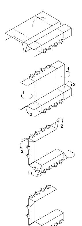
**Stage 1**: With test rig opened out flat and fillings in position, thread cover behind hinge pin and clip to top and bottom of the frame. Raise the larger frame to the vertical position.
