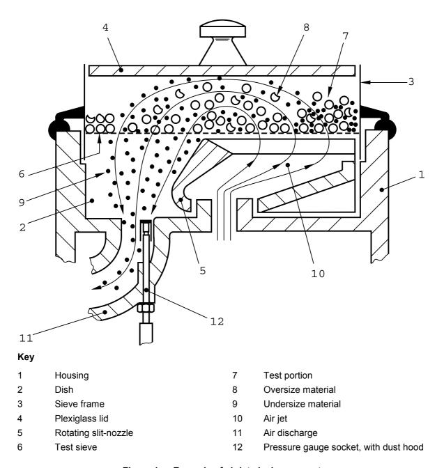
Figure 1 — Example of air jet sieving apparatus
