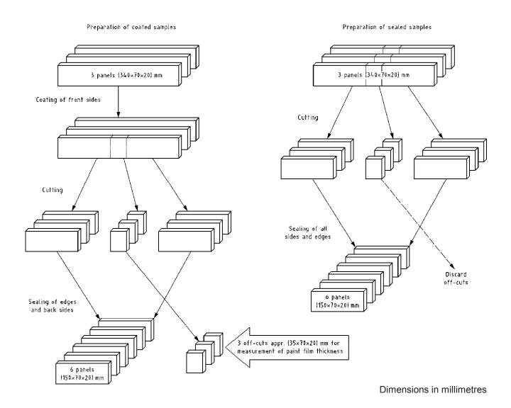
Figure 2 — Cutting of test panels
