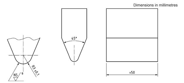
$<sup>^{1)}</sup>$  The roughness grade N5 in accordance with EN ISO 1302 corresponds to a roughness value Ra of 0,4  $\mu$ m.
