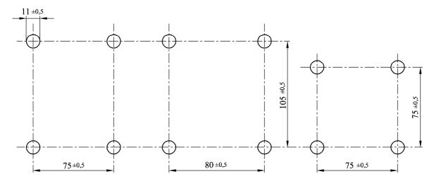
Figure 5 — Distance between centres of castor wheels
