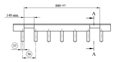
Figure 4 — Frontal receiver with integrated handles
