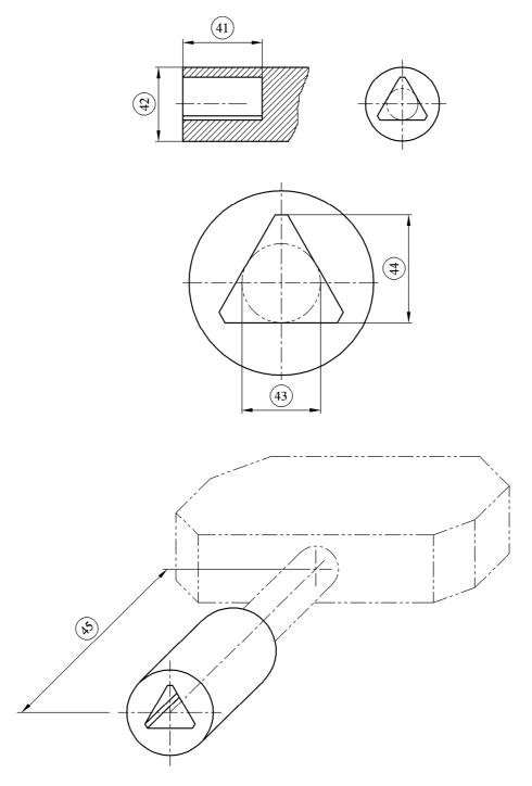
Figure 6 — Standard triangular key
