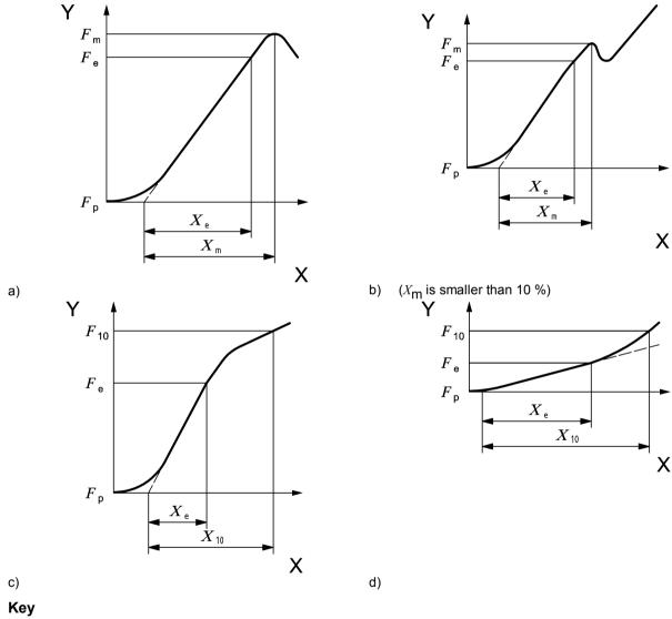
$F_{\rm p}$  force corresponding to the preload  $F_{\rm m}$  maximum force  $X_{\rm m}$  displacement at maximum force  $F_{\rm 10}$  force at 10 % strain  $X_{\rm 10}$  displacement at 10 % strain force corresponding to the preload
