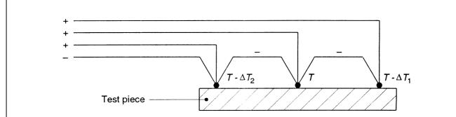
Figure 4 — Example of arrangement of differential thermocouples to monitor temperature distribution in the test piece, where  $\Delta T_1$ ,  $\Delta T_2$  are differential temperatures (see Table 1)
