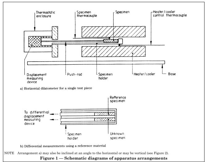
**5.2** Construction materials. For measurements from below ambient temperature to 1 000 °C, transparent fused silica or fused quartz shall be used for construction of the test piece holder. For measurements from ambient temperature to temperatures above 1 000 °C, an alumina ceramic of at least 99,8 %  $Al_2O_3$  shall be used for construction of the test piece holder.
