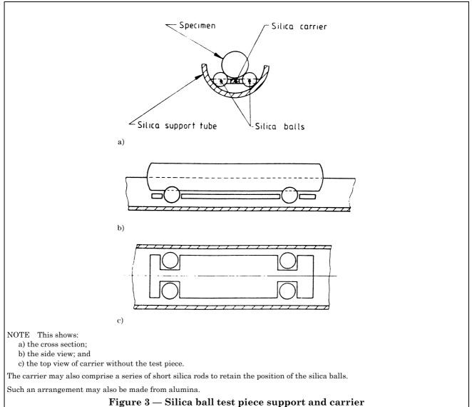
rigure 5 — Sinca ban test piece support and carrier
