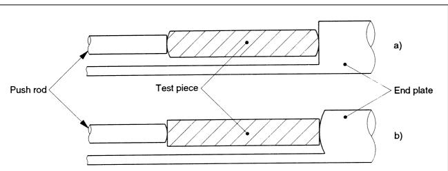
Figure 5 — Test pieces with a) rounded ends for use with flat end plate and push rod surfaces and b) flat square ends for use with rounded end plate and push rod surfaces in a conventional horizontal dilatometer
