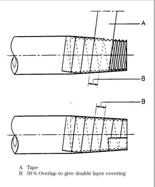
Figure 1. Clock wise wrapping procedure for Class G tapes (coarse threads)
