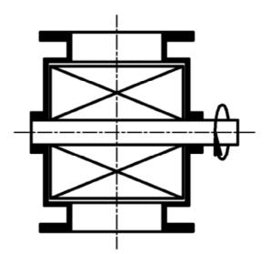
Figure 7 - Example of a typical drop through rotary valve feeder
