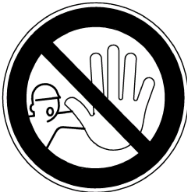
Figure 1 - "Access for unauthorized persons prohibited"
