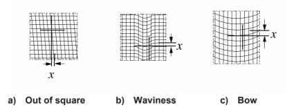
NOTE The scale of these drawings has been exaggerated in order to be explicit about the types of deviation.
