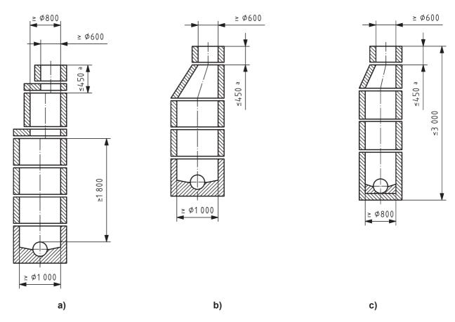
The 450 mm shaft depth (including the straight part of the taper, if applicable) is required to allow the first step or ladder rung to be in an accessible position. For septic tanks or separators, this dimension can be increased up to 600 mm.
