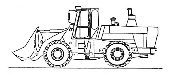
Figure B.1 — Earth and landfill compactors with loading equipment
