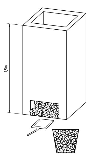
Figure 2 — Hopper and basket, rubber chippings
