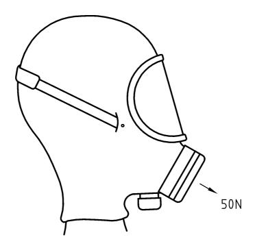
Figure 7 — Scheme of test arrangement for tensile force
