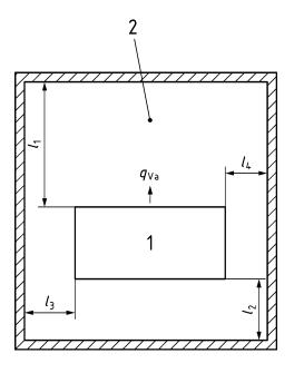
$$\begin{split} &l_1 \geq 1, 5 \times \sqrt{A \times B} \\ &l_3, l_4 \geq 0, 75 \times \sqrt{A \times B} \\ &l_2 \quad \text{according to manufacturer's} \end{split}$$
