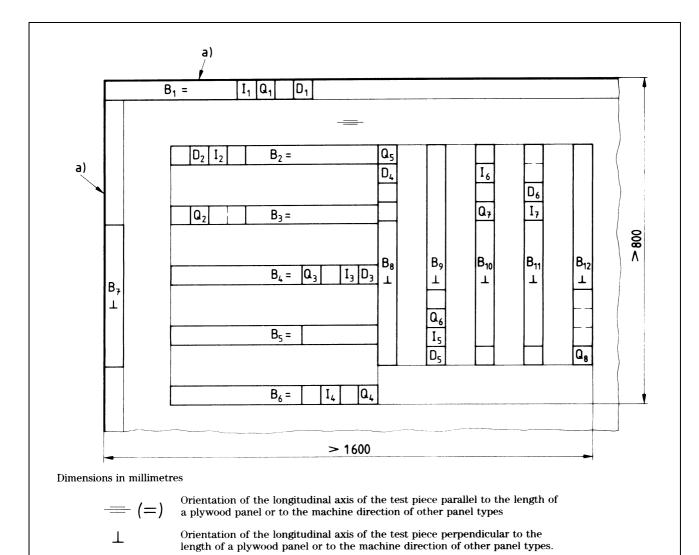
NOTE For properties which are independent from orientation (e.g. D, I and Q) one test piece shall be taken from an outer edge of a trimmed panel where this can be identified.
