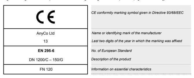
Figure ZA.1 — Example of CE marking on the product for a chamber ring
