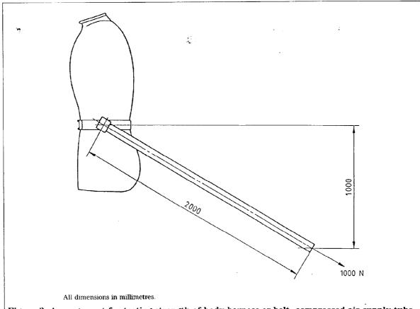
Figure 3. Arrangement for testing strength of body harness or belt, compressed air supply tube and couplings
