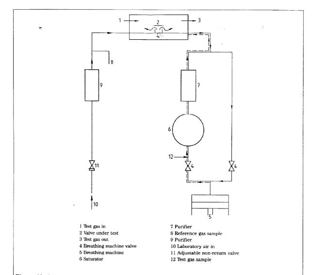
Figure 10. Arrangement for testing exhalation valve leakage using a single cylinder breathing machine
