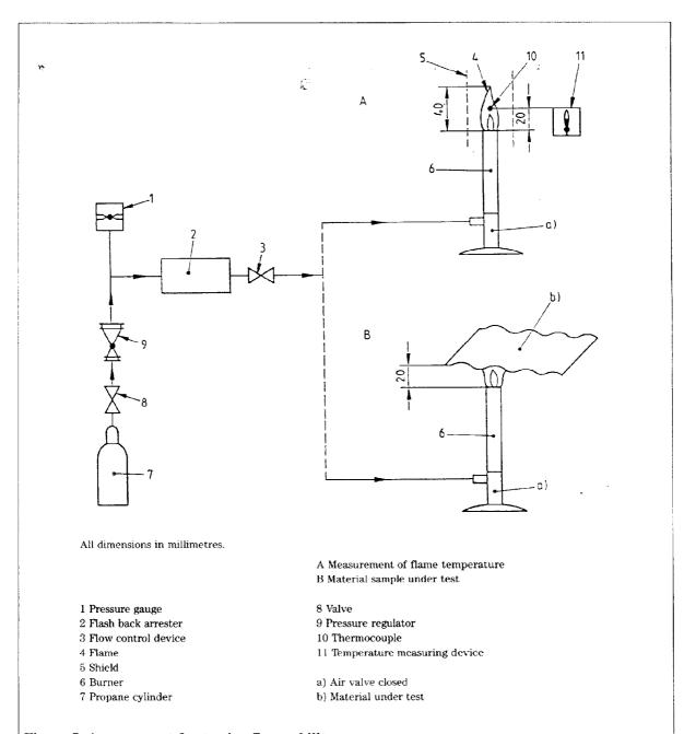
Figure 5. Arrangement for testing flammability
