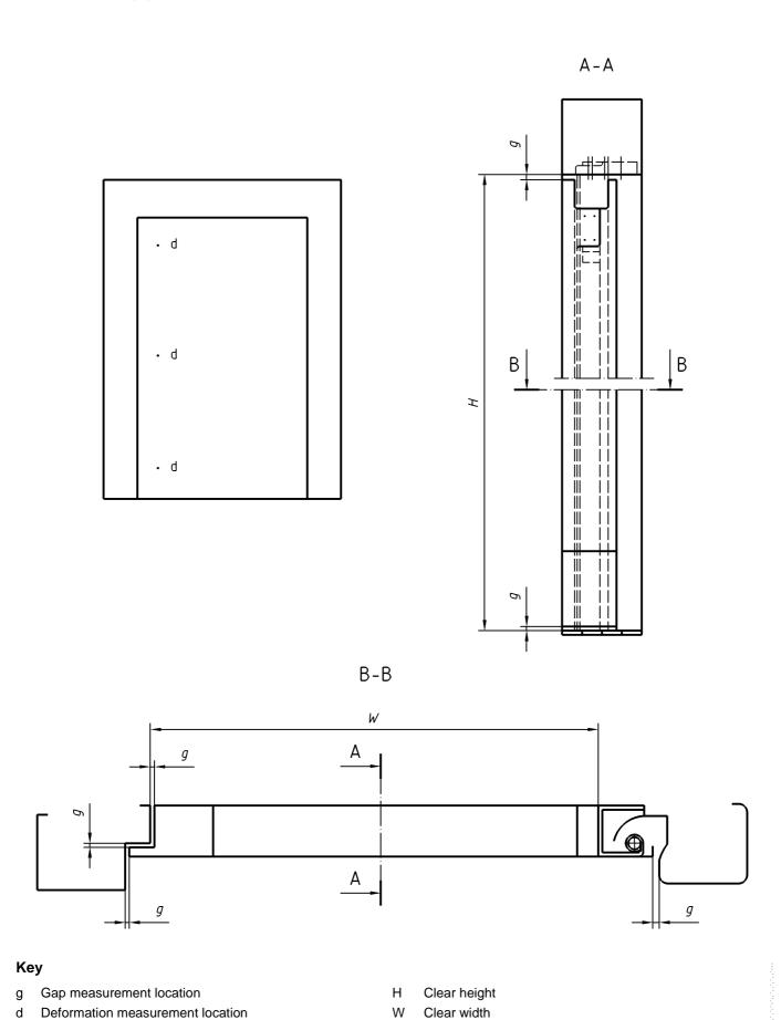
Figure 1 — Clearance gaps (g) and deformation measurements (d) – Single panel swing door
