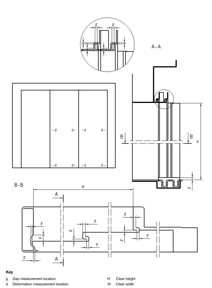
Figure 2 — Clearance gaps (g) and deformation measurements (d) – Double leaf telescopic door
