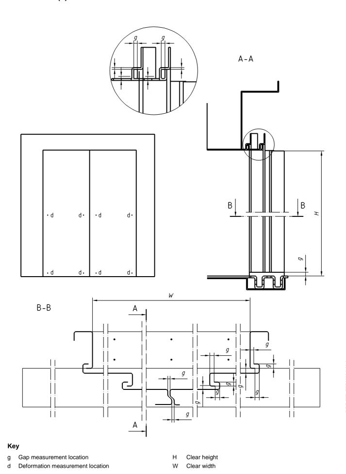
Figure 3 — Clearance gaps (g) and deformation measurements (d) – Central opening door
