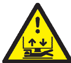
Figure 4 — Warning sign "Pit crush hazard"
