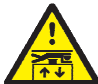
Figure 3 — Warning sign "Overhead crush hazard in lift well"
