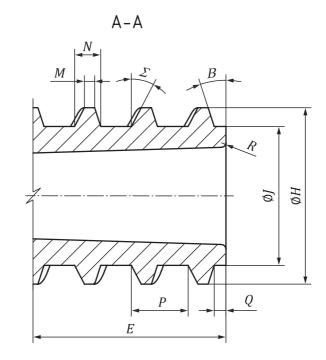
Table B.5 contains the dimensions for this figure. This design and the associated dimensions shall apply to any female LUER LOCK CONNECTOR that has threads in a plane inclined to the axis of the CONNECTOR. There are no dimensional restrictions on thread length. Figure B.6, Figure B.7 and Figure B.8 apply to designs utilizing lugs that are at a right angle to axis of the CONNECTOR.
