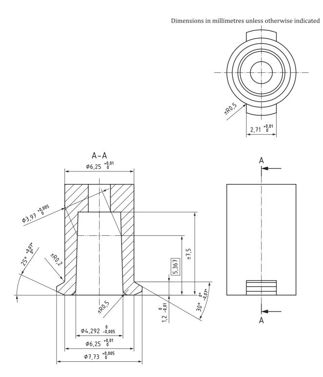
In Figure C.3, all outside edges of lug or thread form shall have a radius between 0,15 mm and 0,20 mm (unless otherwise specified). R may be  $\times$  45° chamfer.
