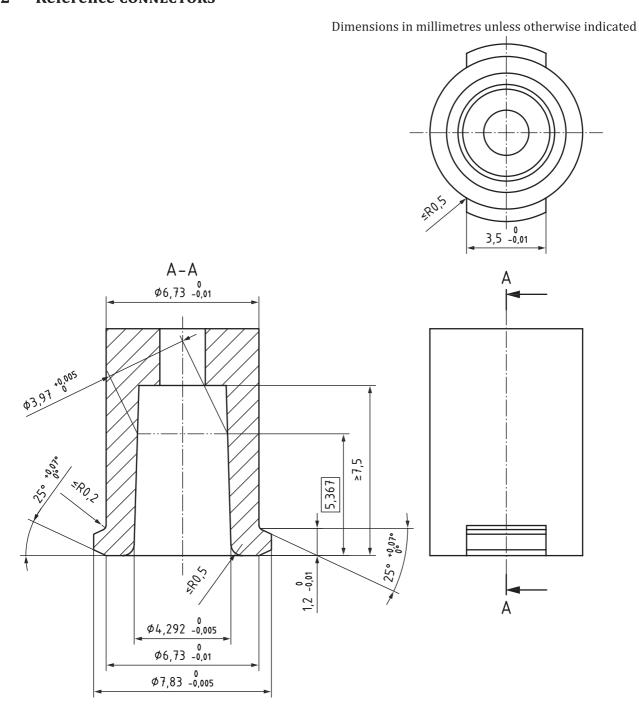
In Figure C.1, all outside edges of lug or thread form shall have a radius between 0,15 mm and 0,20 mm (unless otherwise specified). R may be  $\times$  45° chamfer.
