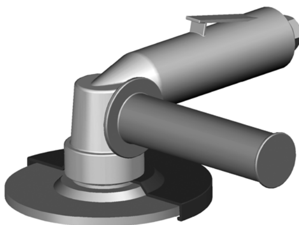
Figure 3 — Pneumatic angle grinder whose motor serves as main handle
