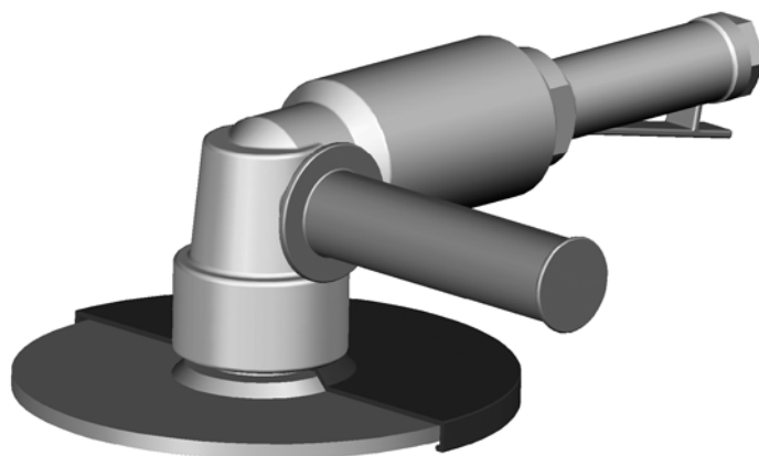
Figure 4 — Pneumatic angle grinder with separate main handle
