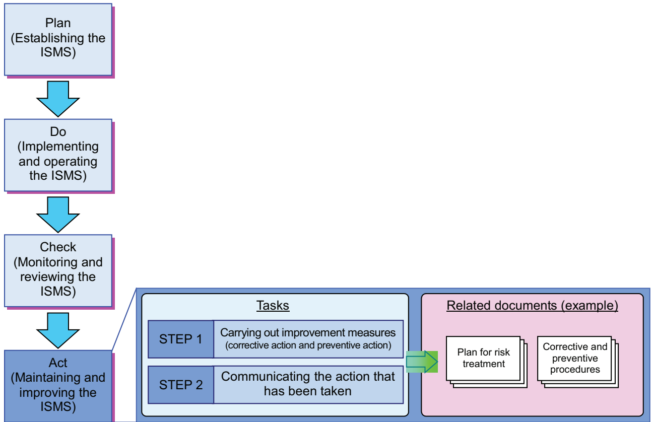
Figure B.7 — Tasks and related documents for monitoring, reviewing, maintaining and improving the ISMS
