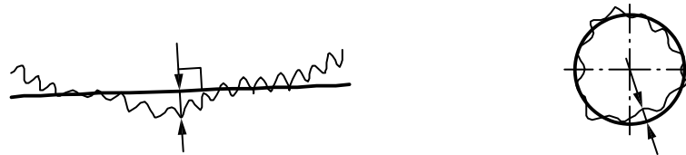
Figure B.15 — Maximum distance between a nominally straight line and a straight line and maximum distance between a nominally circular line and a circle
