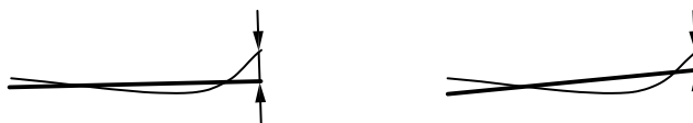
Figure 22 — Independent form characteristic of a nominally straight line with different criteria of association of the corrected line
