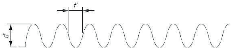
Figure 7 — Measurement of the grid in Figure 6 ; the spacing is measured correctly, but the depth is smaller ( d' < d )
