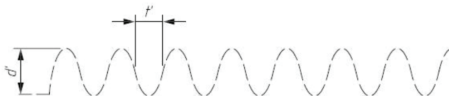
Figure 7 — Measurement of grid in Figure 6 — Spacing measured correctly but depth smaller ( d' < d )
