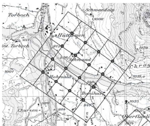
Figure A.10 — Landscape window (LUU) of 1 km 2 with superimposed sampling grid (16 points)
