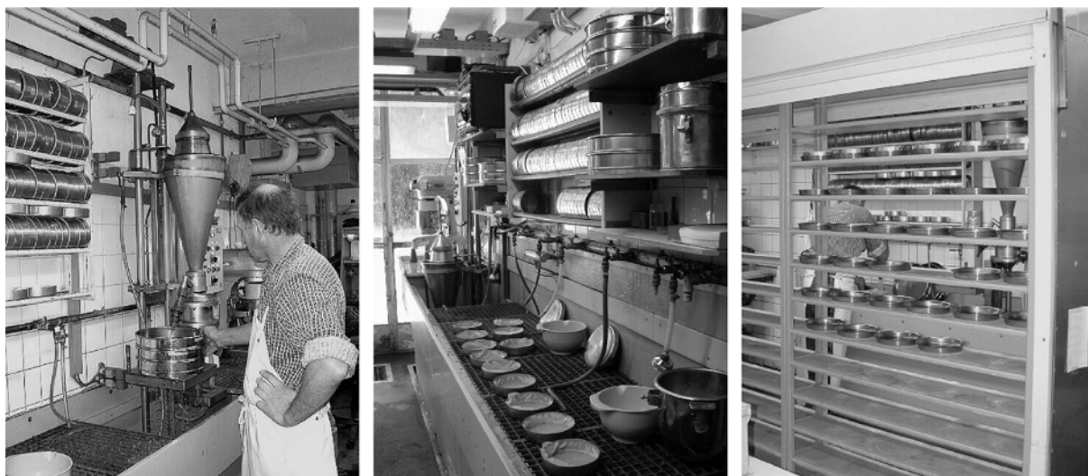
Figure A.5 — Automated Oostenbrink funnel for routine analysis (left), extraction sieves with filters (middle) and rack with extraction dishes (right)
