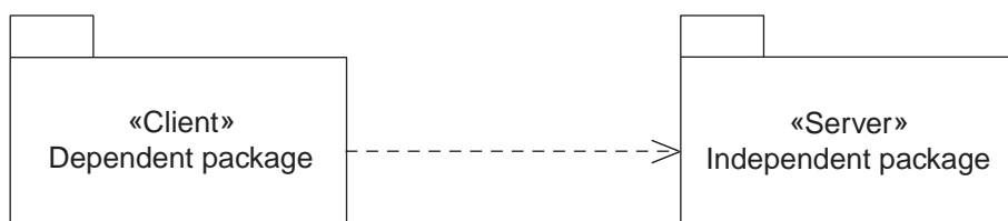
Figure 2 — UML example package dependency
