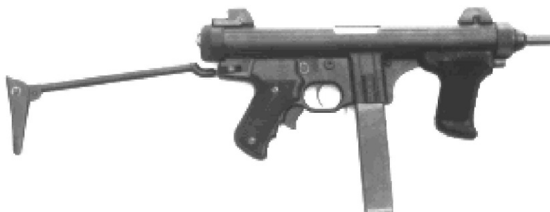
Figure A.14 — Submachine gun with blow-back action
