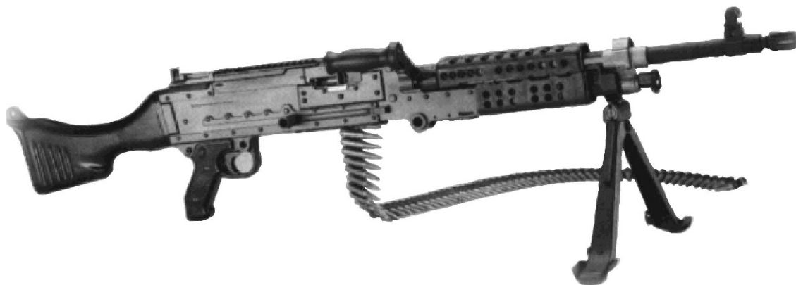
Figure A.16 — Machine gun with locked breech action
