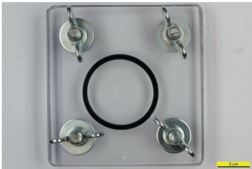
Figure C.2 — compression of O-ring using 4 screws
