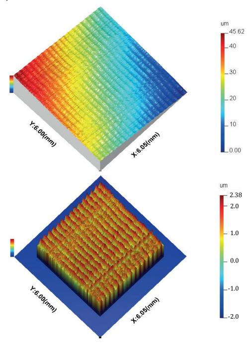
NOTE Top is the original surface, bottom is the filtered surface.
