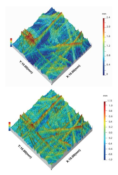
NOTE Top is the original surface, bottom is the filtered surface.
