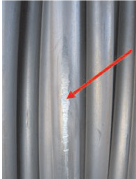
Figure C.1 — Abrasive damage caused by coil-to-coil contact
