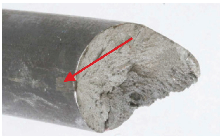
Figure C.4 — Mechanical damage on the rod surface (indicated by an arrow)
