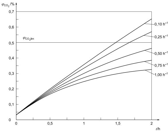
$\begin{array}{lll} \textbf{Key} & & & \\ \varphi_{\text{CO}_2} & & \text{CO}_2 \text{ volume fraction} \\ & t & & \text{time} \\ & & \varphi_{\text{CO}_2,\text{lim}} & \text{AGW value (Arbeitsplatzgrenzwert; maximum workplace atmosphere limit value, 5 000 ppm, TGRS 900} \end{array}$
