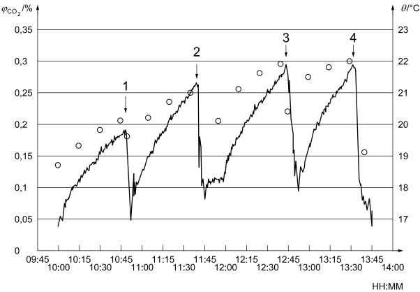
Figure 2 — CO<sub>2</sub> measurement in a school with 5 min rapid air change by opening door and window in the breaks after a 45 min lesson. The room volume was 155 m<sup>3</sup> and during the lesson there were 28 people in the room (Reference [19])
