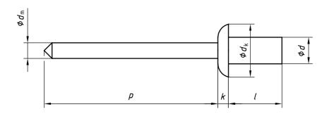
Figure 1 — Rivet dimensions
