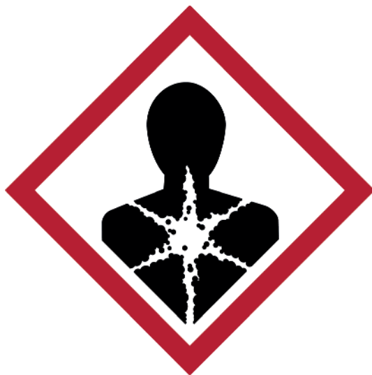
Figure 3 — STOT RE1 pictogram for indicating presence of silica powder at concentrations above 1 % mass fraction
