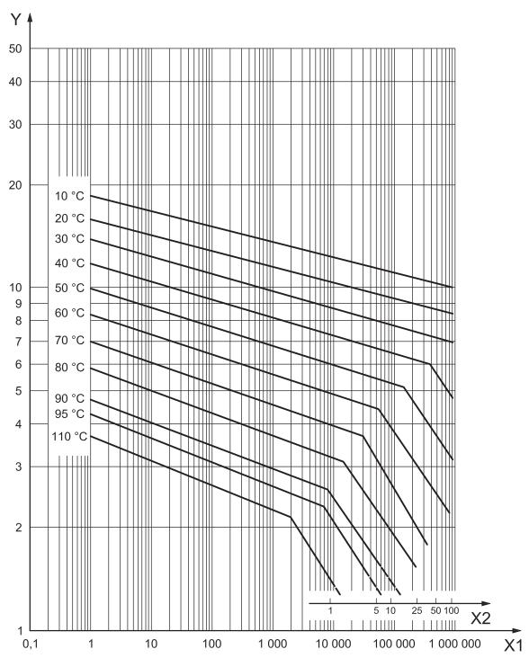
KeyX1time,  $t_1$ , to fracture, in hoursX2time,  $t_2$ , to fracture, in yearsYhoop stress,  $\sigma$ , in megapascal
