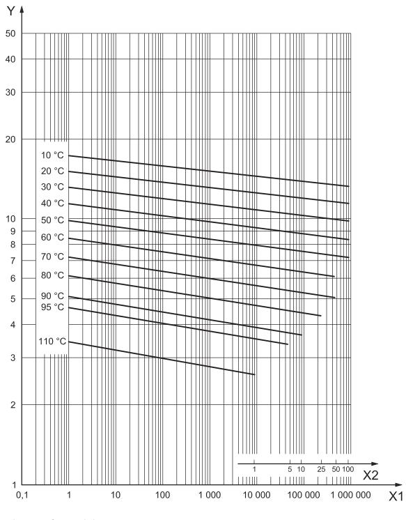
$\begin{array}{lll} \textbf{Key} \\ \textbf{X1} & \text{time, } t_1 \text{, to fracture, in hours} \\ \textbf{X2} & \text{time, } t_2 \text{, to fracture, in years} \\ \textbf{Y} & \text{hoop stress, } \sigma \text{, in megapascal} \\ \end{array}$
