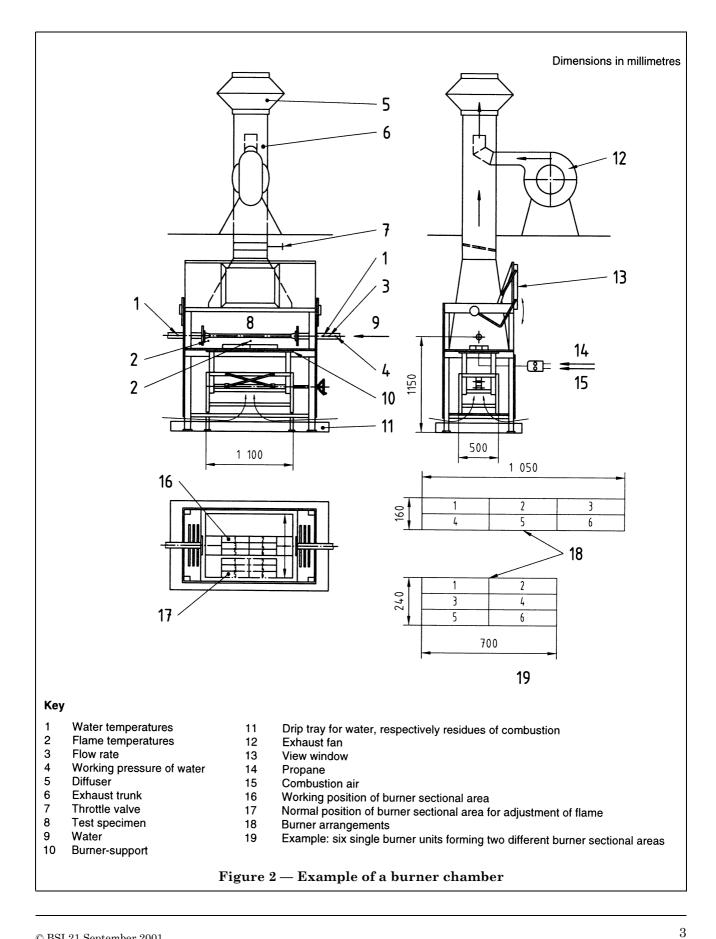
The burner shall be movable to avoid exposing the test piece to the flames during adjustment of the flame.
