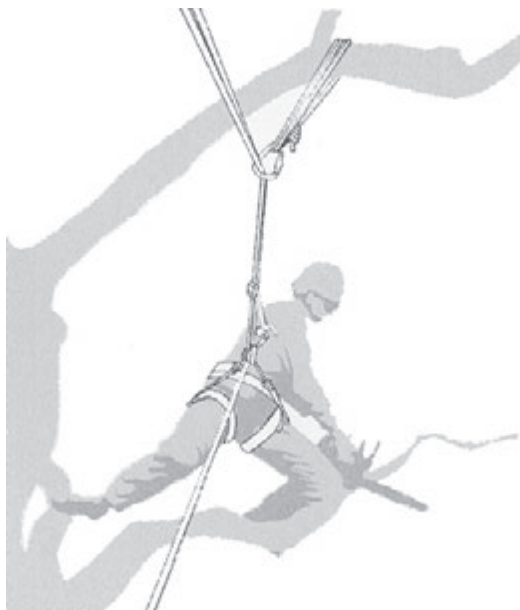
Figure A.3 — Example of redirection of main line via supplementary anchor point
