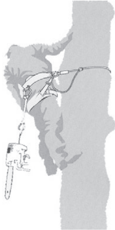
Figure A.2 — Example of attachment of tree service chain-saw to centre rear mid-point on harness
