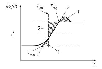
dQ/dt heat flow rate T temperature 1, 2, 3 areas between DSC trace and baselines (see 10.1.4) a Endothermic direction.
