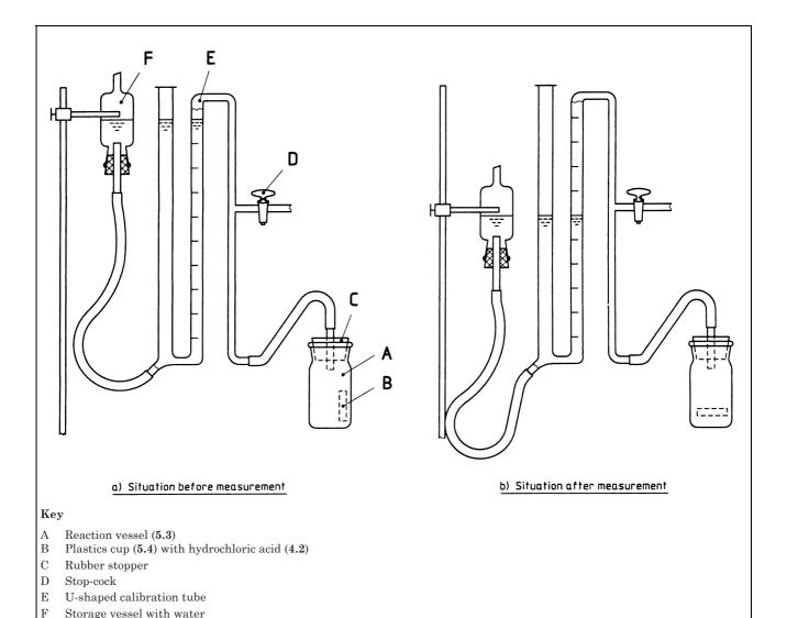
Figure 2 — Example of a single Scheibler unit
